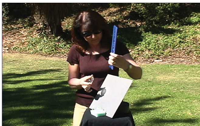
Fig. 2. A still image of video 1: Measuring the focal length of a convex lens using the sunlight and a ruler.
